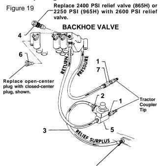
For John Deere Tractors use reservoir plug. Remove plug, drill with 37/64 drill, and tap 3/8 NPT pipe. Screw plug onto hose, locking with Locktite to assure assembly will remain together during connecting and disconnecting procedures. Obtain another plug from your dealer to use when backhoe is removed.
